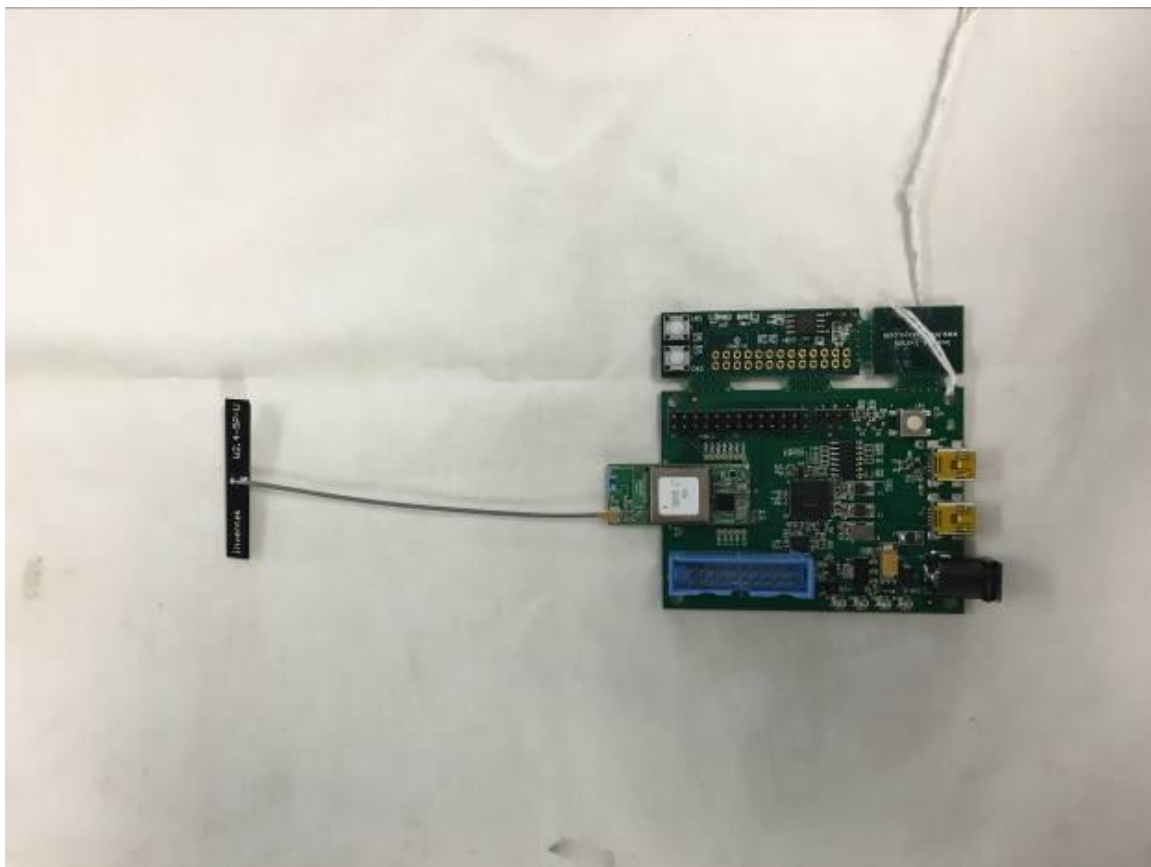
Figure 5. Radio Module on EVB Carrier Board (this configuration only supports WiFi+BT)
