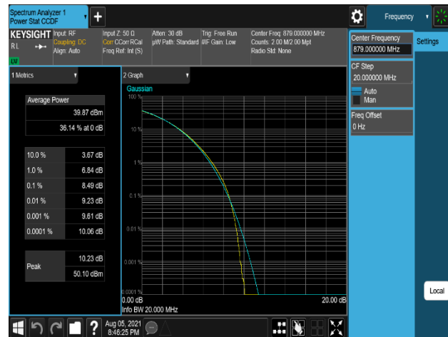
Plot 7-288. Peak To Average Power Ratio Plot (DSS_B5_10M+10M_2C_QPSK - Low Channel, Port 3)
