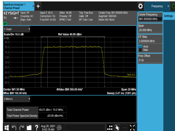
Plot 7-231. Conducted Average Output Power Plot (DSS_B5_10M_9:1)_1C_64QAM - Mid Channel, Port 1)
