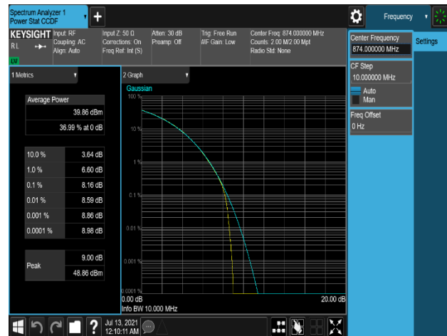
Plot 7-269. Peak To Average Power Ratio Plot (LTE_B5_10M_1C_256QAM - Low Channel, Port 0)
