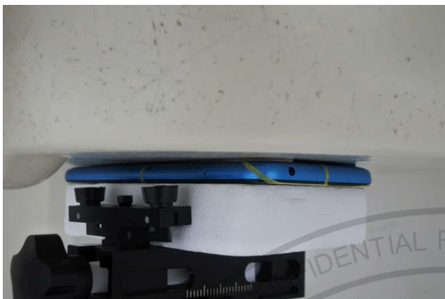
Back, Test Separation 0 mm
