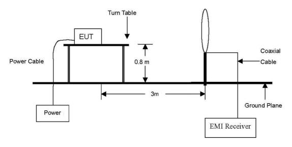
The diagram below shows the test setup that is utilized to make the measurements for emission from 30 Mb to 1 @ Emissions.
