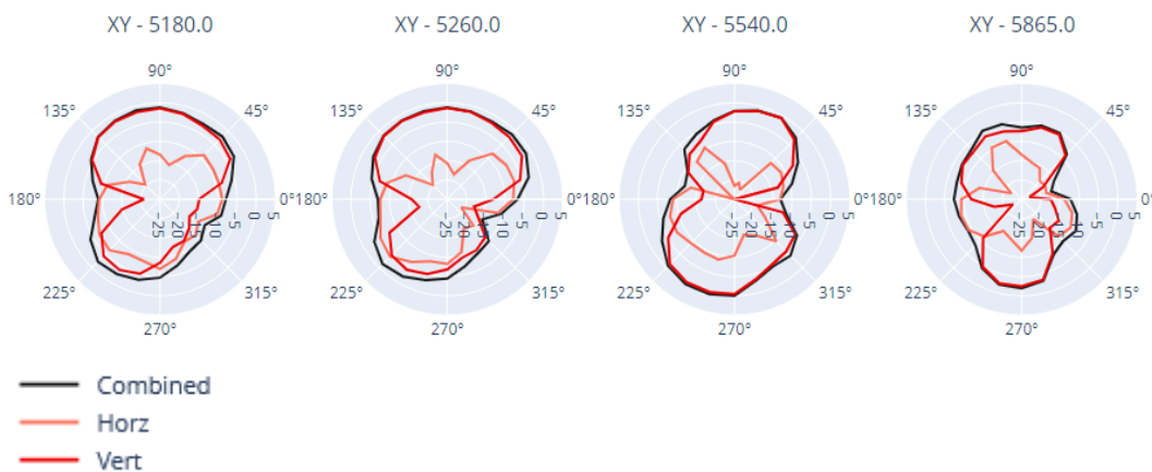
Figure 5: AFG4507W2S-0200S antenna – 5 GHz, 2D X-Y plane radiation pattern
