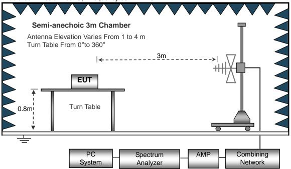
(C) Radiated Emission Test-Up Frequency Above 1GHz
