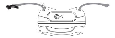
The receiver can be moved on the nylon strap to make it even tighter.
