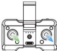
Simultaneously push the left joystick and the right joystick to the bottom right corner to calibrate the gyro. The indicator lights on the drone will blink and turn solid, and the transmitter will send out a long “Di” sound, which indicates the calibration is completed.
