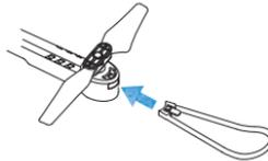
As shown in the picture, install the propeller guard to the motor base.
