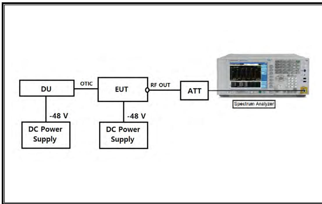
**SETUP DIAGRAM FOR TESTS (RADIATED TEST SETUP)**
