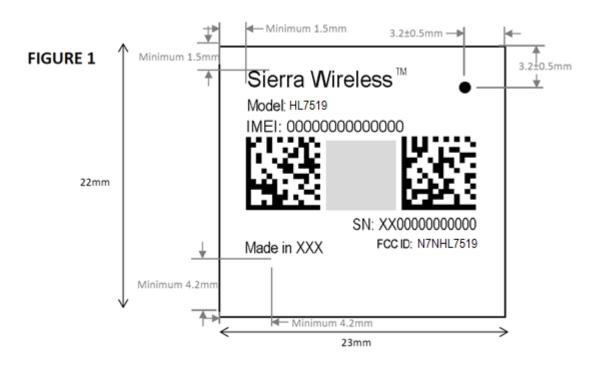
Dimensions are taken with respect to the edge of the surface that the laser etch is made on.
