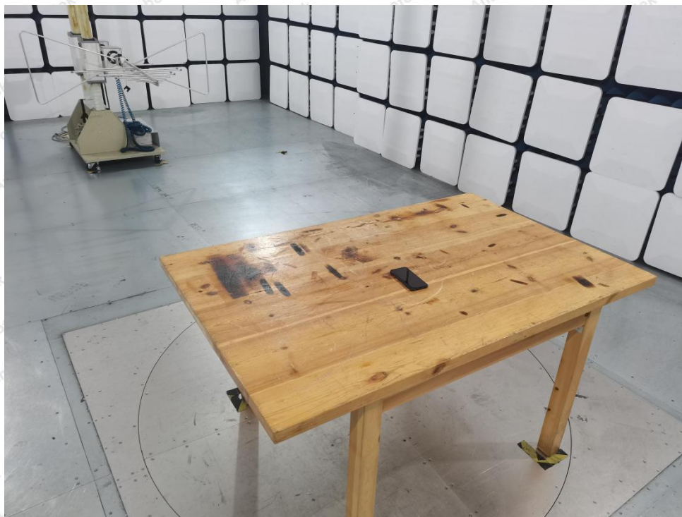
Photo of Radiation Emission Test
