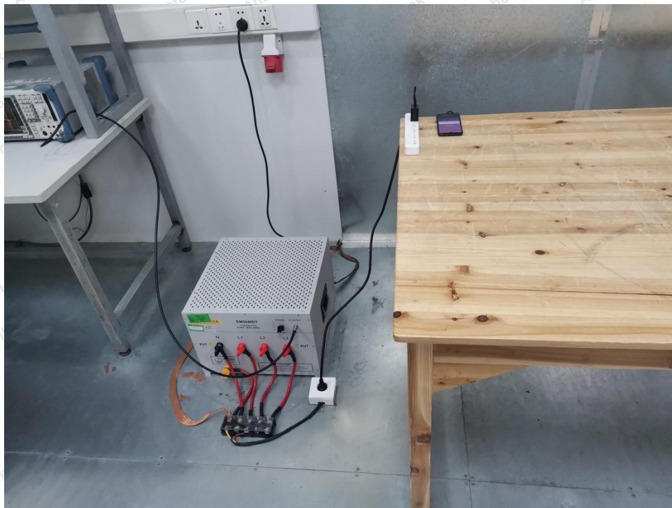
Photo of Conducted Emission Measurement
