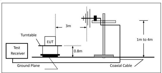
(c) For radiated emissions above 1000MHz
