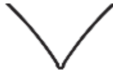
Offset is too high: bubbles appear at the corners
