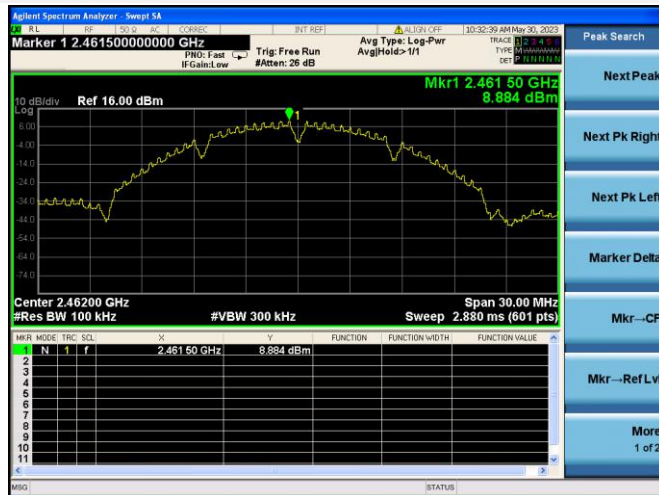
802.11b HIGH CHANNEL, CARRIER LEVEL
