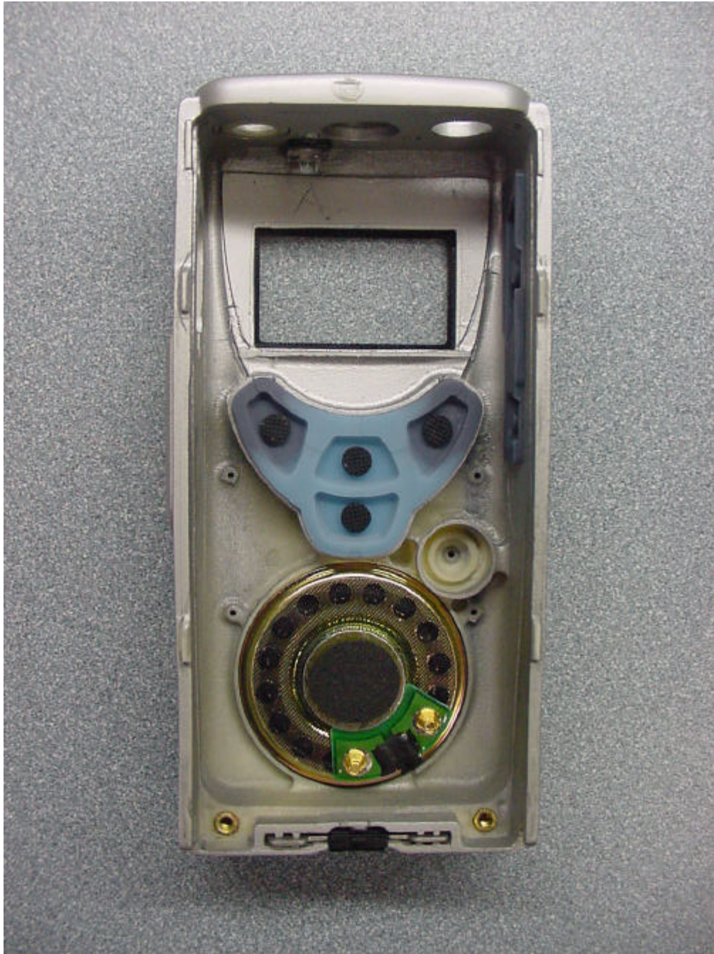
PHOTOGRAPH 13: INSIDE OF FRONT COVER (MURS-25)
