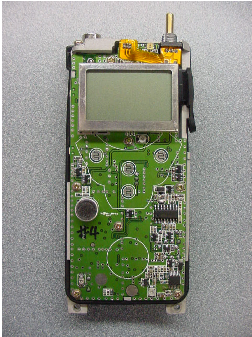
PHOTOGRAPH 12: FRONT OF PCB MOUNTED INSIDE CHASSIS (MURS-25)
