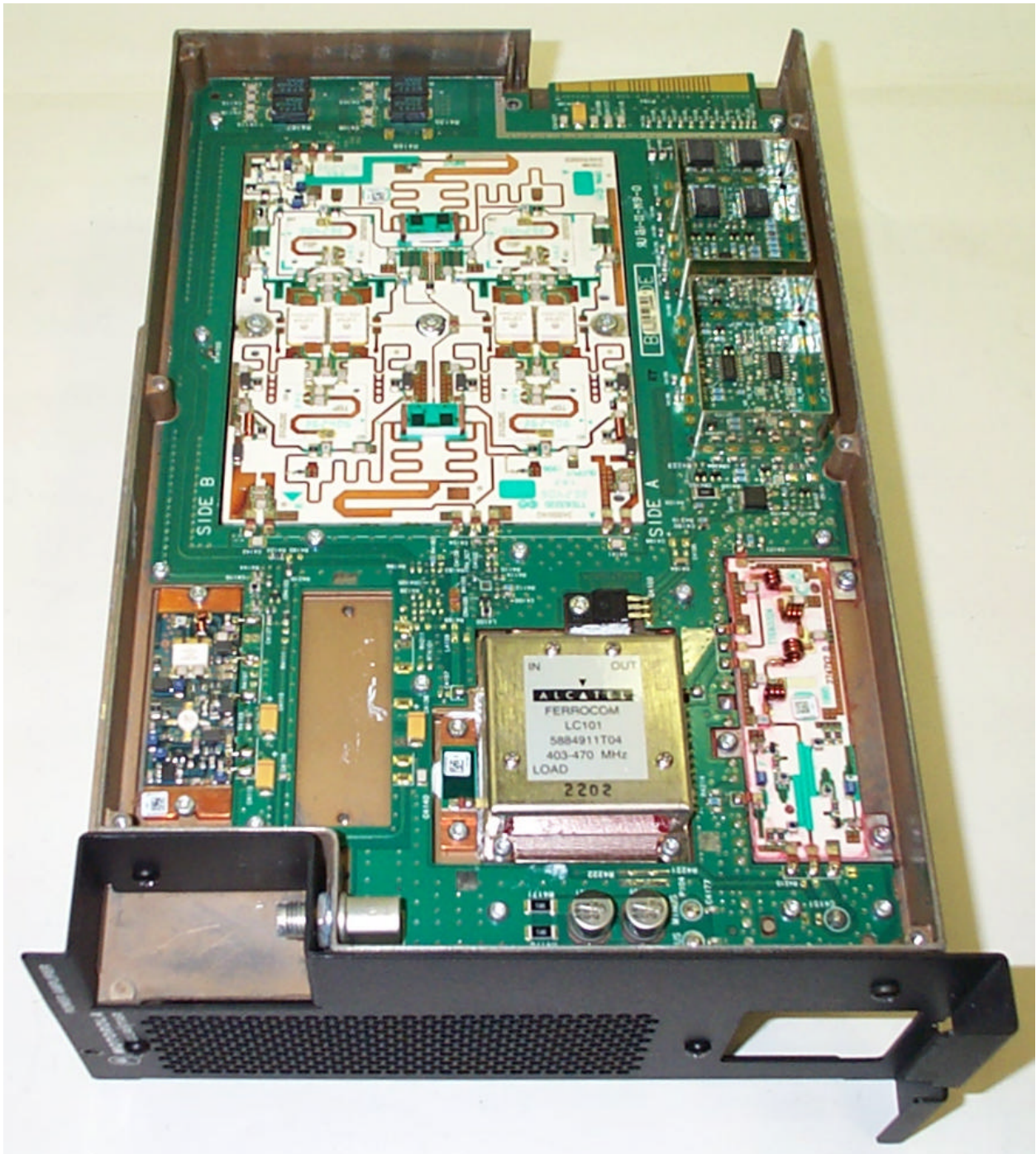
Power Amplifier Module, Top View, Shields Removed – Range 2 PA Shown
