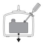
Set 2X1.5V battery in the correct direction.
