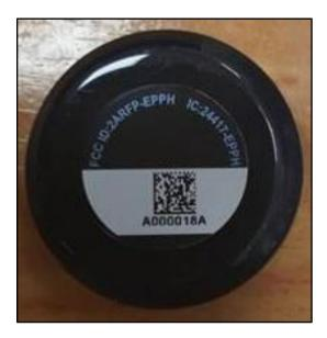
Label with **FCC ID: 2ARFP-EPPH and IC: 24417-EPPH** will be located here. The statement according to FCC part 15 §15.19(a)(3) is placed in User Manual, page 4 (Application exhibit User\_manual\_40972).
