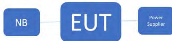
Fig. 2-2 Conducted (Antenna Port) Emission Configuration
