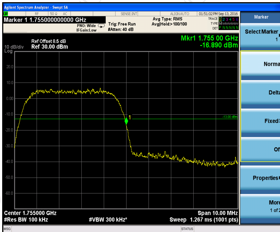
Higher Band Edge Plot on Channel 1513
