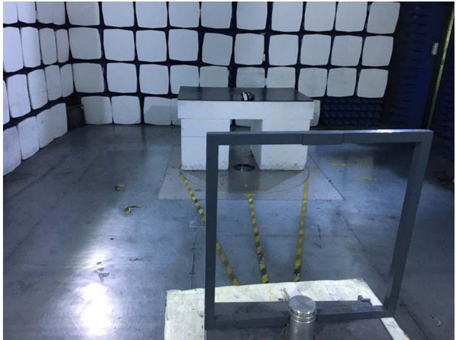
Radiation Emission Test Setup (Below 30MHz)
