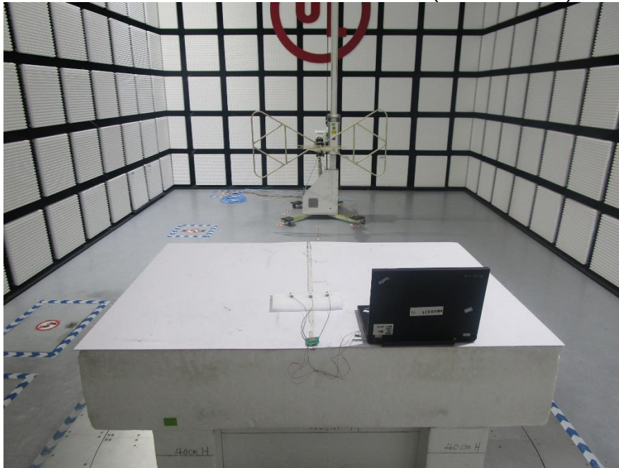
RADIATED RF MEASUREMENT SETUP (30MHz~1GHz)
