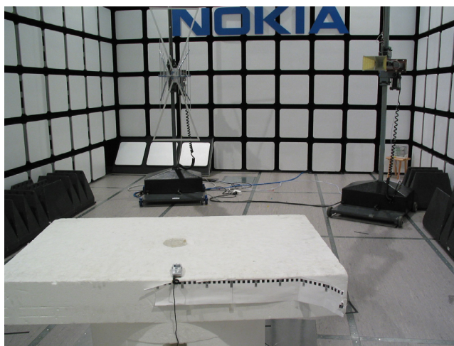
Picture 5 EUT test setup, flip closed
