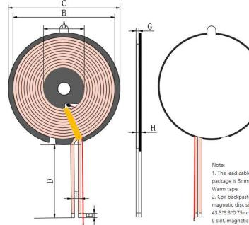
Note: 1. The lead cables are crossed. The outlet package is 3mm wide and high
