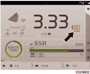
The icon will be orange and the load will not be locked if the system can't weigh the load because one or more of the previously described conditions are not met.
