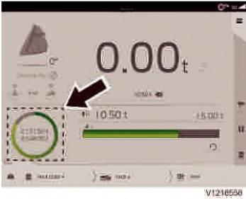
Shows fulfilment of the target load for the active work order. The green part of the circle shows added load. The target load has been reached when the circle is completely yellow. In case of overload, a notification in red will show the overload in number of tonnes. Tap on the circle to edit and finish the active work order.
