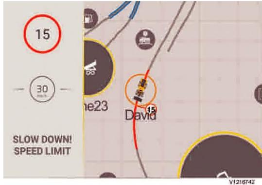
Some roads where the machines/vehicles operate may be so narrow that there is only room for one at a time. When the map is created it is possible to add single-lane roads. When two machines/vehicles are approaching the same single-lane road, warnings will be shown.
