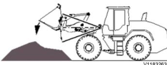
(back to pile). Only tap on the message if the dumped material should be added in the system.
