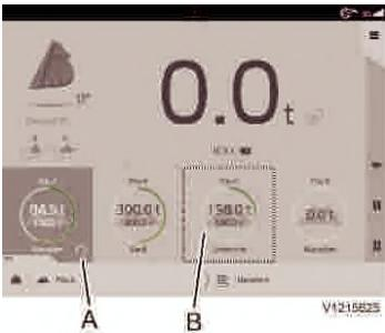
In pile mode, fulfilment of the target load to piles are shown. The green part of the circle shows added load. The target load has been reached when the circle is completely green.
