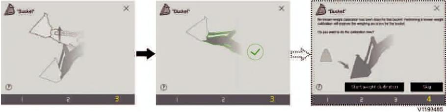
Lift with a smooth continuous lifting motion all the way up to the target position. To keep the lifting speed constant, it is recommended to use full lever stroke and the engine in idling speed all the way up to the target position where the confirmation is given. If the system does not accept a step it will indicate how to redo that step.
