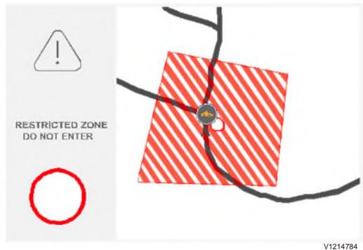
There may be prohibited zones on the site, as well as no-vehicle zones, for example where the ground is too soft or a zone is at risk of collapse. These zones may be marked and warnings may appear on the screen when the machine/vehicle enters the zone.
