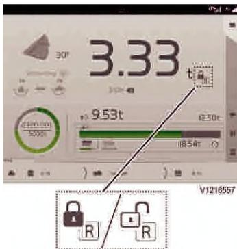
Padlock (locked / unlocked weight)
