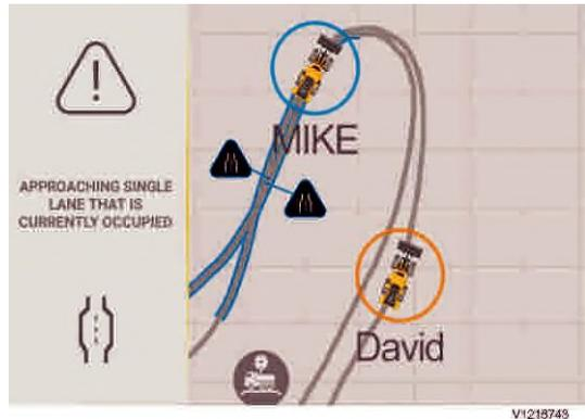
When another machine/vehicle is on a single-lane road farther ahead.
