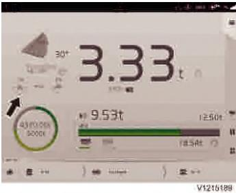
Shows the angle for transversal inclination.
