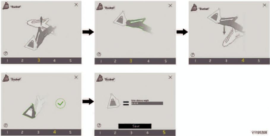
Follow the guidance in the display. Lift with a smooth continuous lifting motion all the way up to the target position. To keep the lifting speed constant, it is recommended to use full lever stroke and the engine at idling speed all the way up to the target position where a confirmation is given. Also lower at a low constant speed all the way down to the target position until the confirmation is given.
