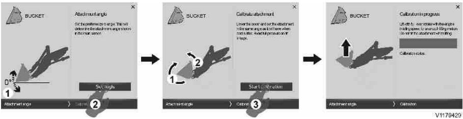
1. Tilt the attachment to the angle preferred as zero angle.
