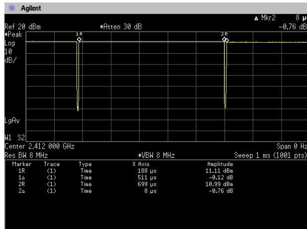
$$\text{Duty Cycle} = T_{\text{on}} / (T_{\text{on}} + T_{\text{off}}) = 511[\text{us}] / (511[\text{us}] + 8[\text{us}]) = 98.5[\%]$$
