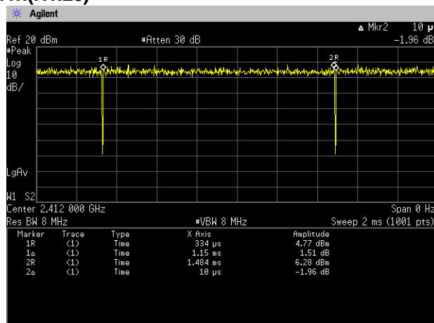
$$\text{Duty Cycle} = T_{\text{on}} / (T_{\text{on}} + T_{\text{off}}) = 1150[\text{us}] / (1150[\text{us}] + 8[\text{us}]) = 99.1[\%]$$
