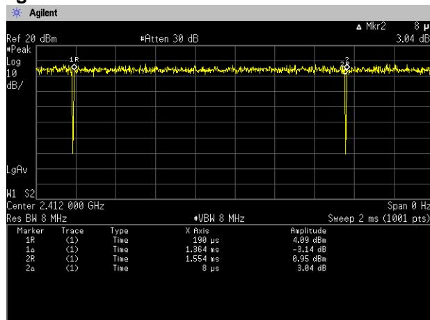
$$\text{Duty Cycle} = T_{\text{on}} / (T_{\text{on}} + T_{\text{off}}) = 1364[\text{us}] / (1364[\text{us}] + 8[\text{us}]) = 99.4[\%]$$
