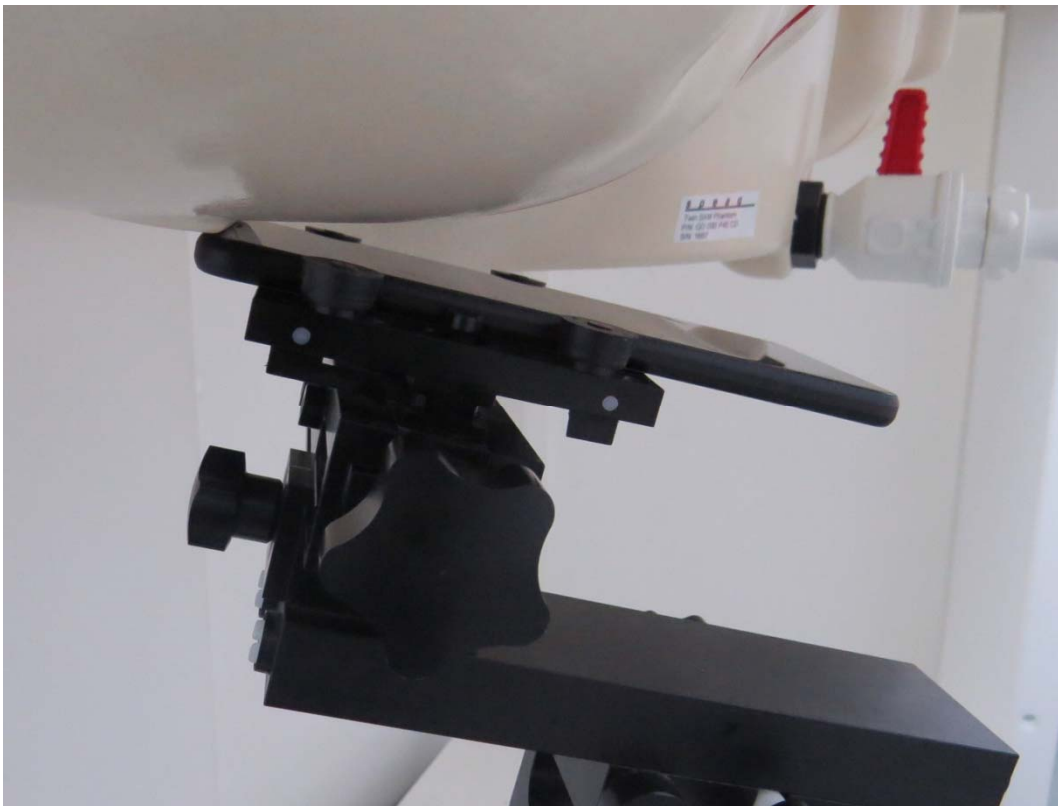
Picture 4: Right Hand Tilt 15 Degree Position
