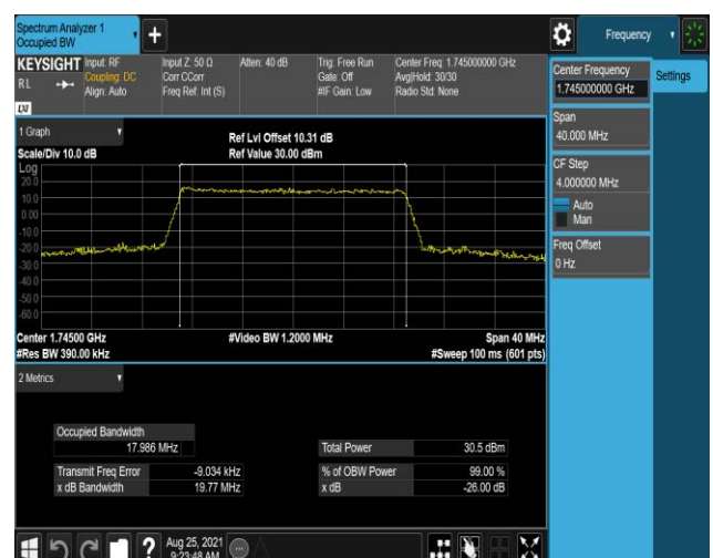
Band4-20MHz-16QAM-20300-100RB#0
