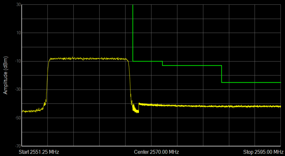
Band7 QPSK BW=15MHz Channel=21375 RB Size=75 Position=#0
