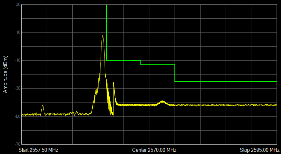
Band7 16QAM BW=10MHz Channel=21400 RB Size=1 Position=#Max
