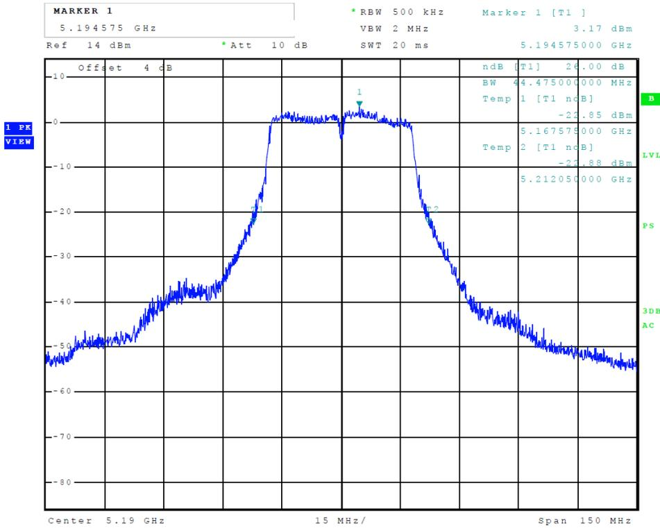
Figure 21 Plot of Transmitter Emissions (Chain 0, 5150-5250 MHz Band, 802.11n40, 26 dB OBW)
