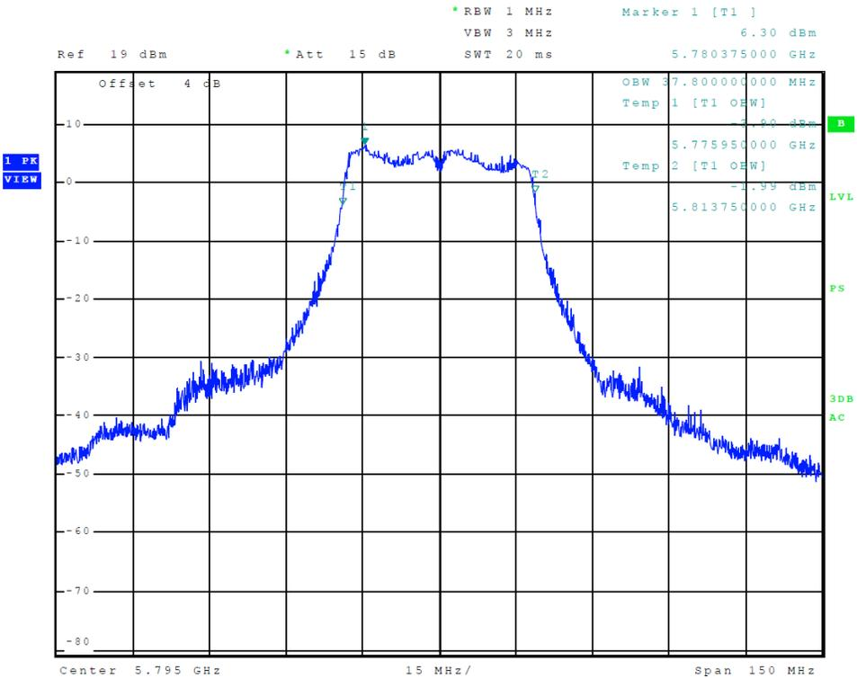
Figure 39 Plot of Transmitter Emissions (Chain 1, 5725-5850 MHz Band, 802.11n40, 99% OBW)
