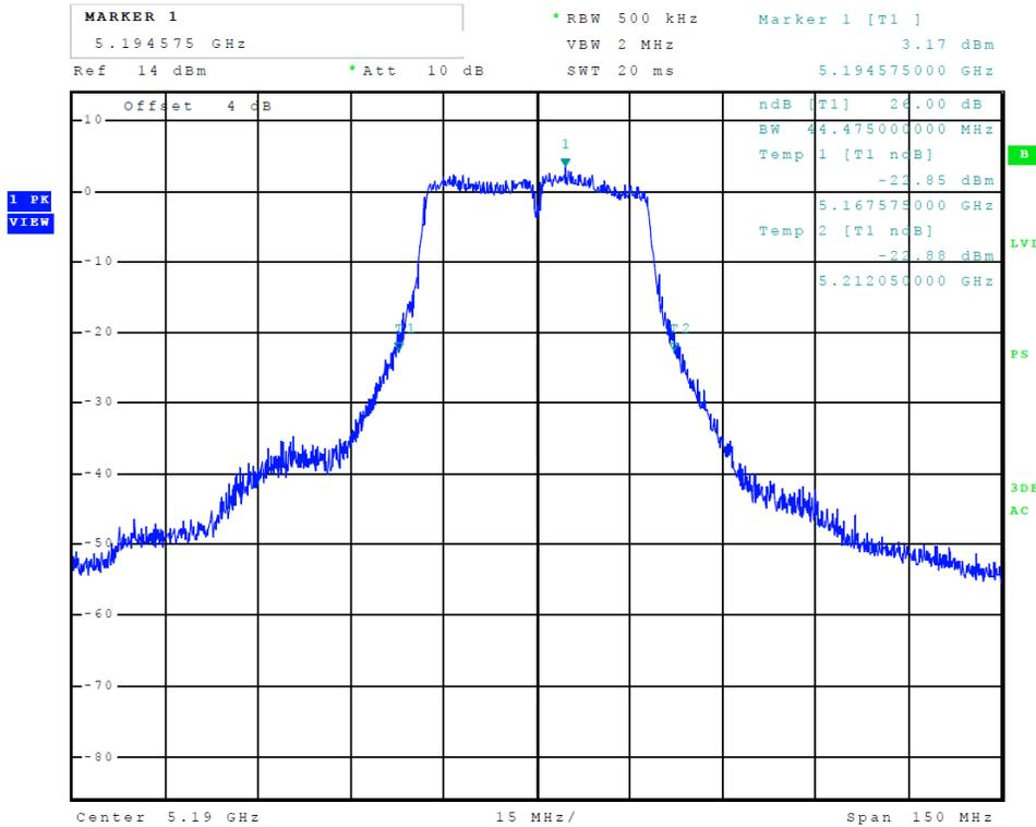
Figure 19 Plot of Transmitter Emissions (Chain 0, 5150-5250 MHz Band, 802.11a, 26 dB OBW)
