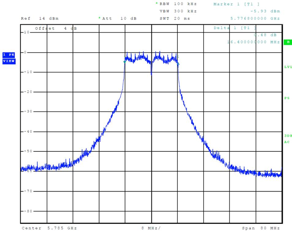
**Figure 39 Plot of Transmitter Emissions (Chain 0, 5725-5850 MHz Band, 802.11a, 6-dB OBW)**
