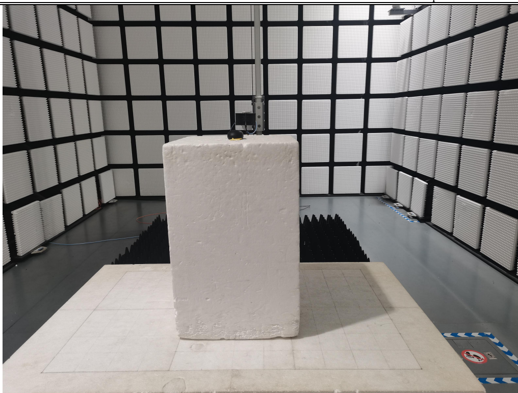
Fig. 3 Radiated emission setup photo(Above 1GHz)
