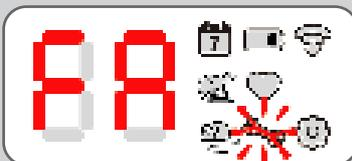
The motor will be tested to ensure it is in working order, this is done first without moving the gate, if the motor is "Not detected" a flashing Service Mode (Icon 🔧) will illuminate and 'FA' (FA) will be displayed. Hold the button down for the failure reason.
