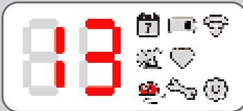
Fifth press of the button will display the Mouse (Icon
