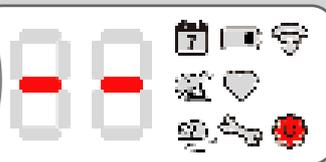
To deploy the unit press and hold the button for three seconds until two dashes (
