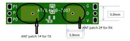
ANT patch 1# and ANT patch 2#, having the same size, make up the antenna system of EUT. Refer to above table and picture for the dimensions of antenna of EUT.
