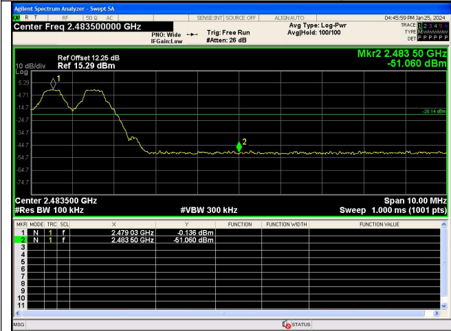
Out Of Band Emission(Right) GFSK_DH5_Channel Hopping
