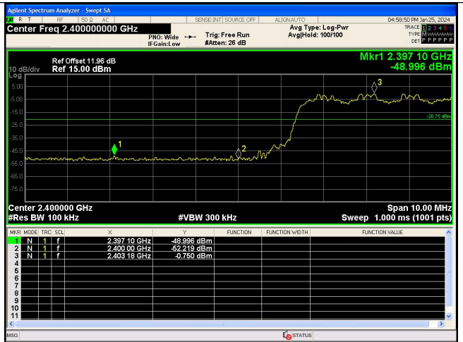
Out Of Band Emission(Left) \pi/4 DQPSK_2-DH5_Channel Hopping
