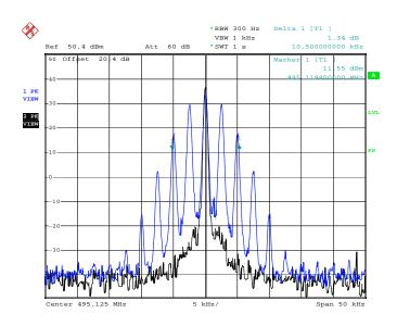
Occupied Bandwidth CS:25KHz Date: 18.OCT.2005 14:33:06
