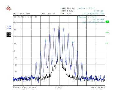
Occupied Bandwidth CS:25KHz Date: 18.OCT.2005 14:28:49
