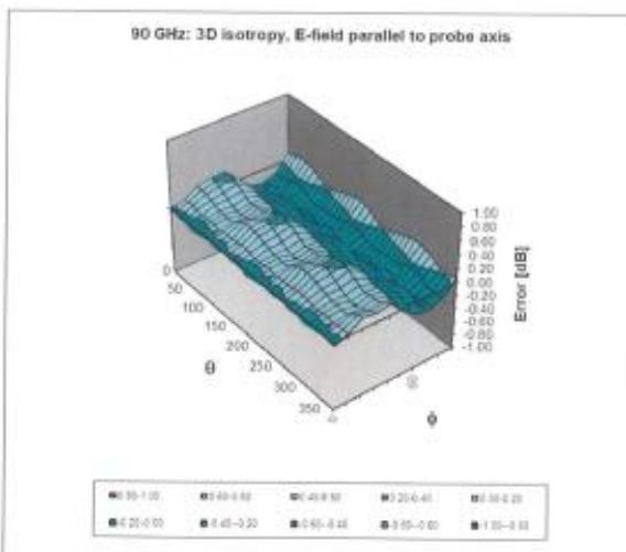
Probe isotropy for  $E_{\text{ext}}$ : probe rotated  $\varphi = 0^\circ$  to  $360^\circ$ , tilted from field propagation direction  $\hat{k}$
