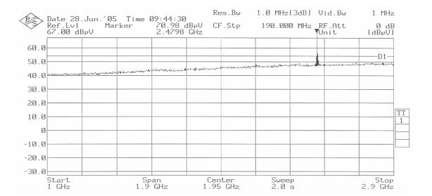
Note: The peak above the limit is the carrier frequency.
