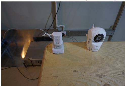
Radiated Emissions (30MHz-1GHz) Test Setup
