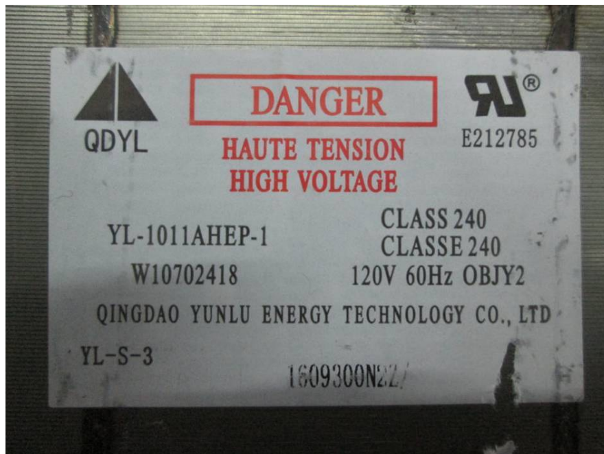
EUT – Transformer Label View
