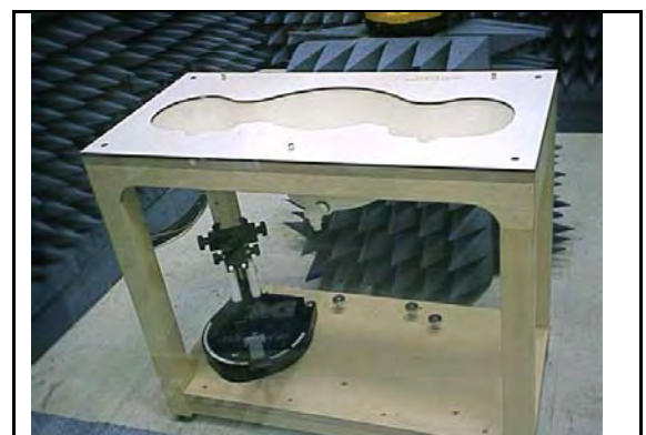
Figure 6. SAM Twin Phantom
