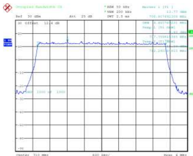
Figure 6-17a: Occupied Bandwidth, Band 5 Middle Channel, 5MHz BW, RB=25
