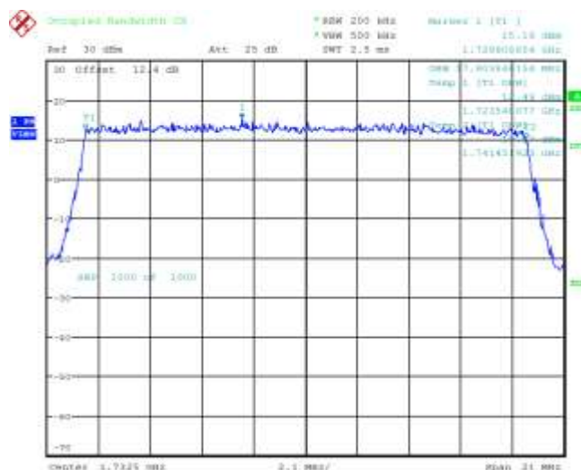
Figure 5-20a: Occupied Bandwidth, Band 4 Middle Channel, 20MHz BW, RB=100
