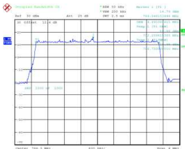
Figure 3-12a: Occupied Bandwidth, Band 5 High Channel, 5MHz BW, RB=25
