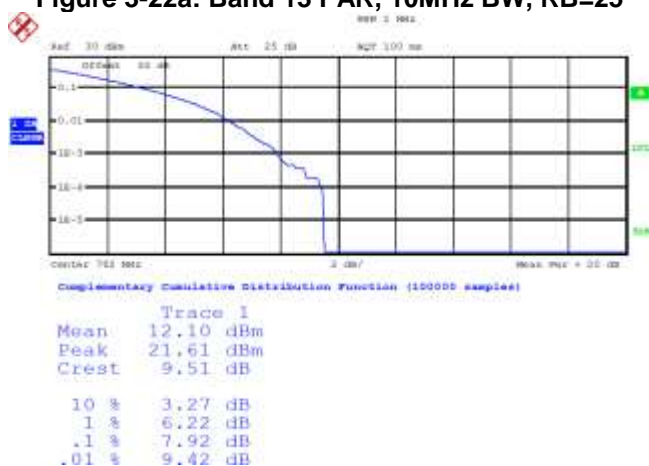
Figure 3-22a: Band 13 PAR, 10MHz BW, RB=25
