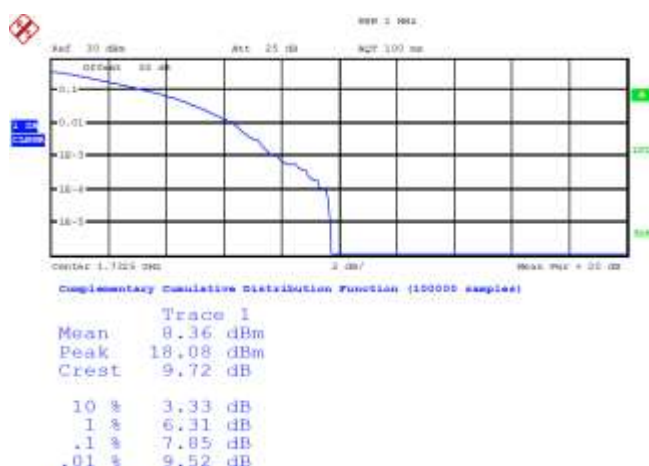
Figure 5-45a: Band 4 Mid Channel PAR, 20MHz BW, RB=50, QPSK
