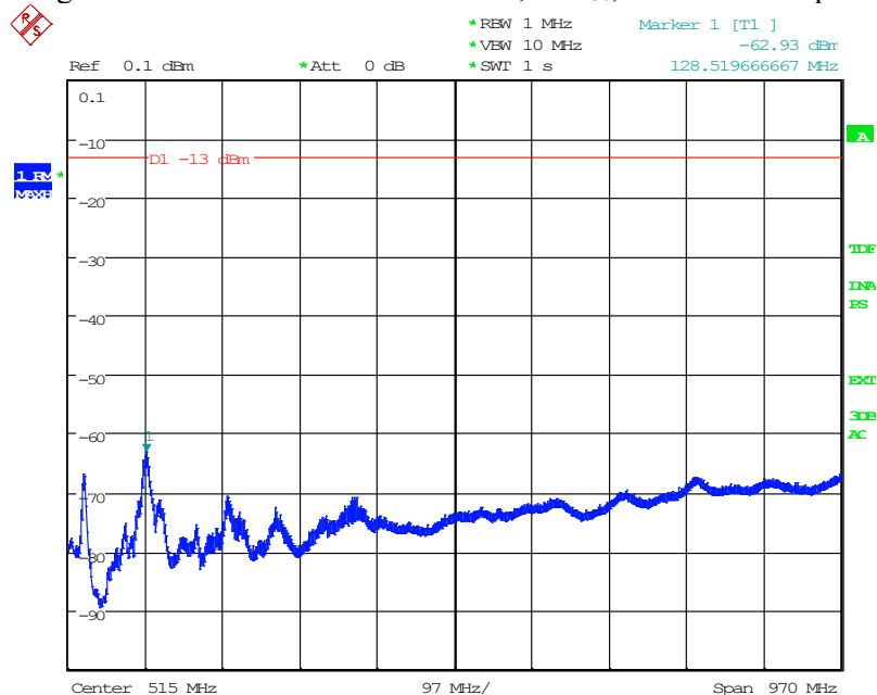
Diagram 2.1b: Pre scan 30 – 1000 MHz, BL 250 , EIRP Vertical polarization
