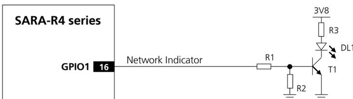
Figure 38: Application circuit for network indication provided over GPIO1
