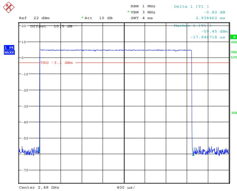
**EDR ( $\pi/4$ -DQPSK):****Pulse time, Low Channel, 2DH1**
