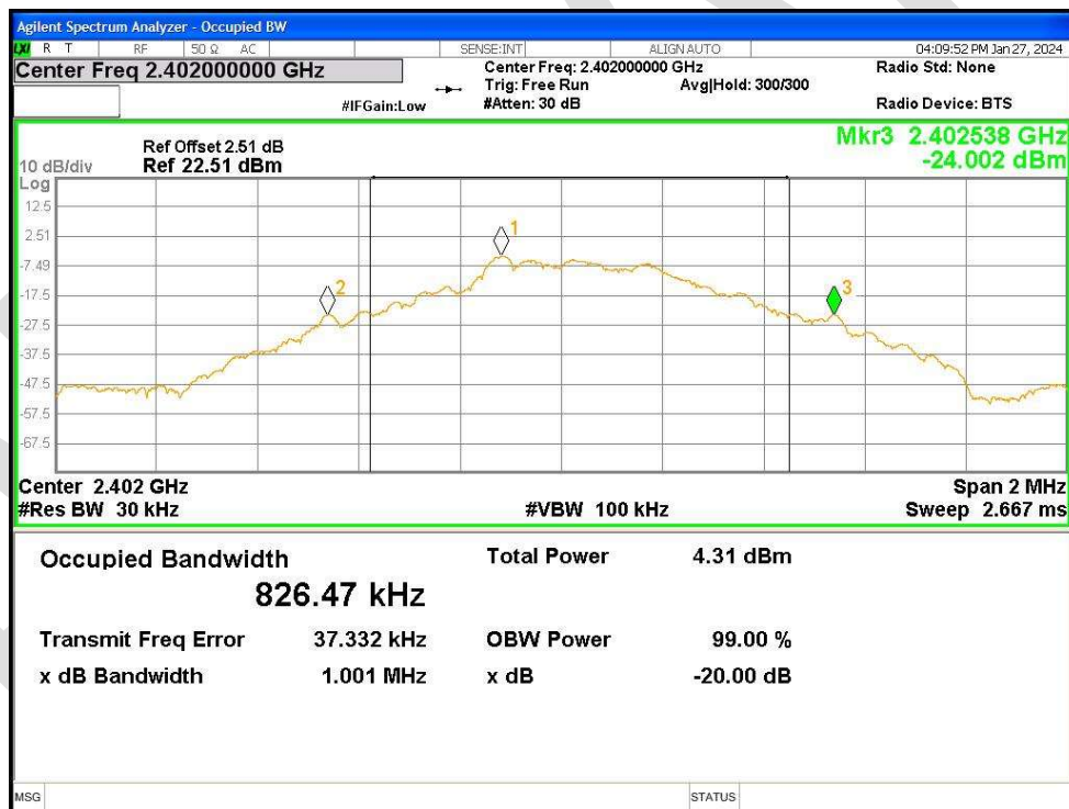
-20dB Bandwidth NVNT 1-DH1 2402MHz Ant1
