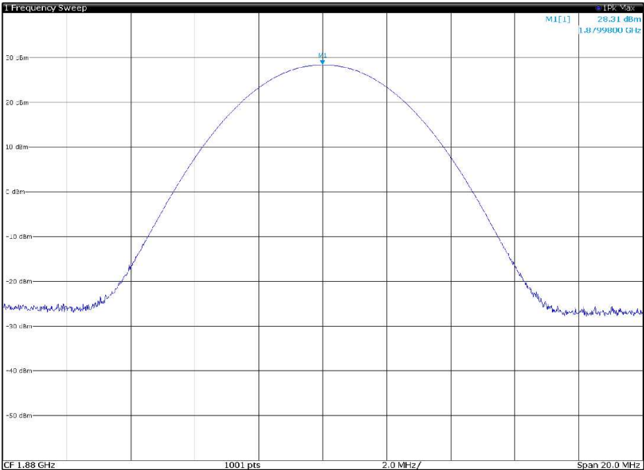
Figure 8.1-17: Output power of GSM 1900, channel Mid
