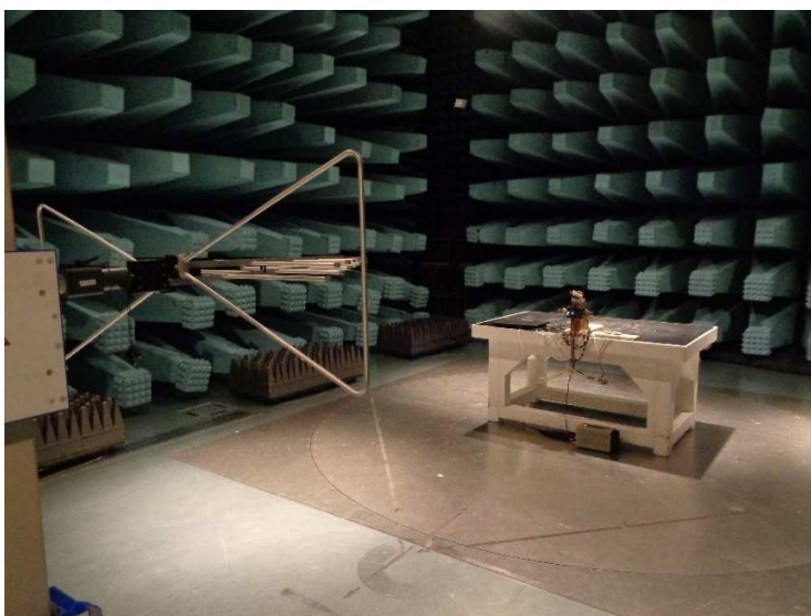
Radiated emission below 1 GHz
