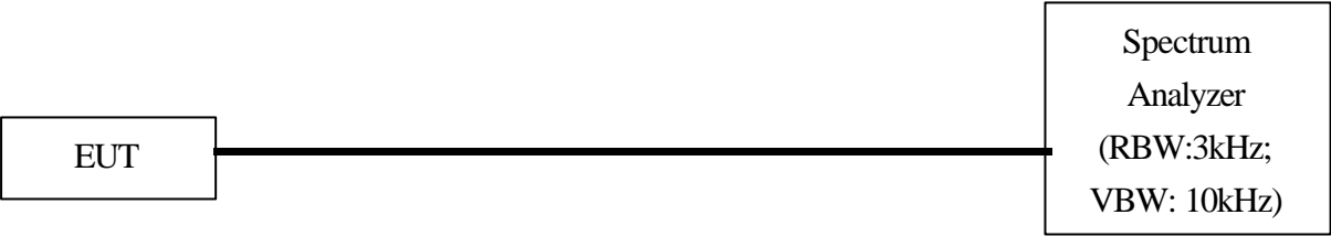
Test Configuration of Power Spectral Density
