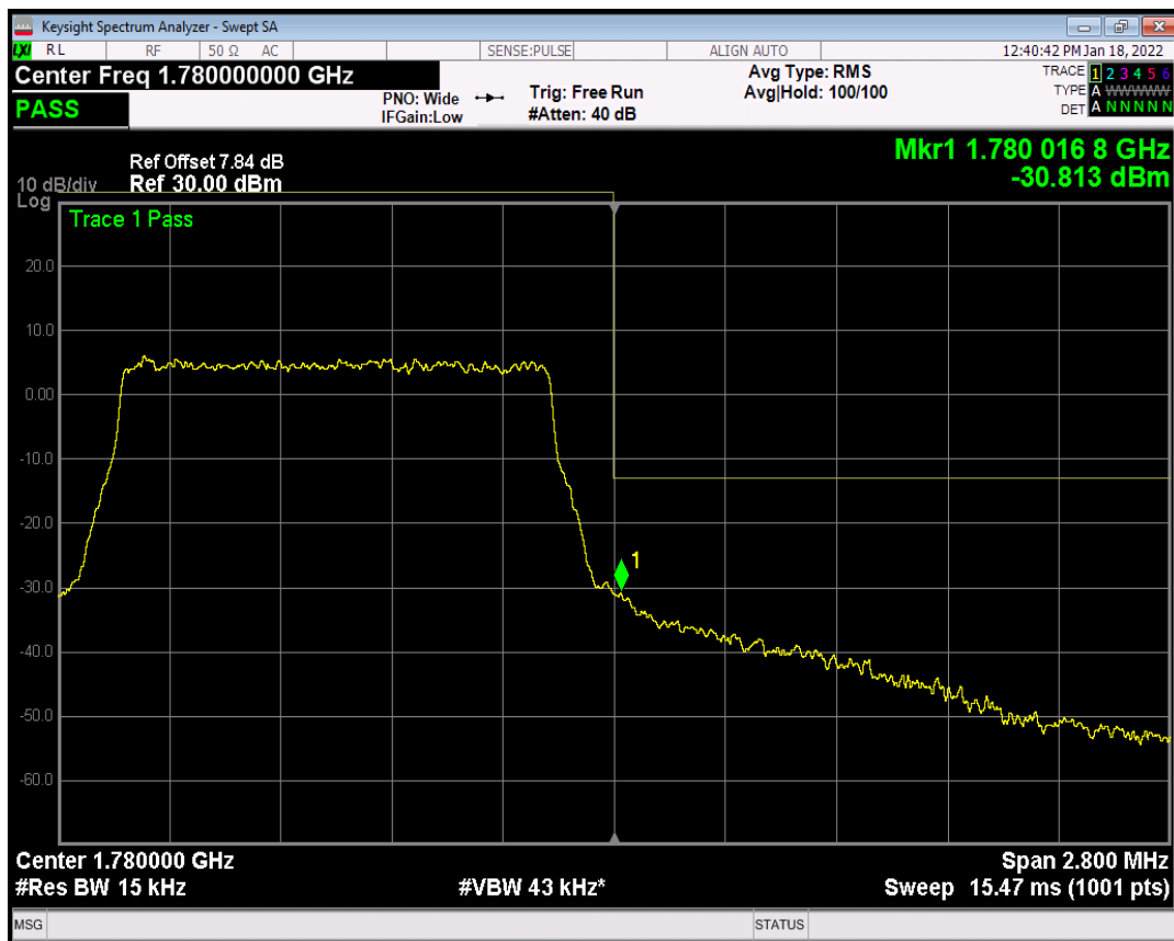
Band66 QPSK BW=10MHz Channel=132622 RB Size=1 Position=#0
