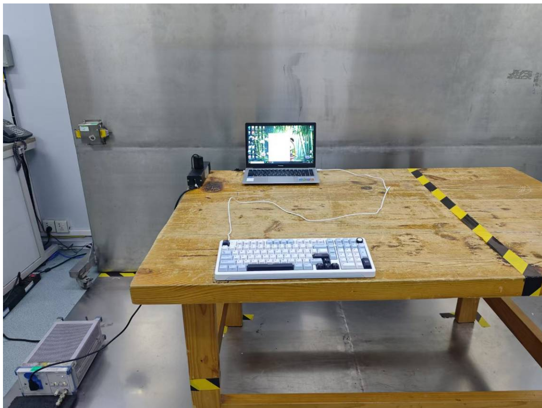
Conducted Emissions Side View
