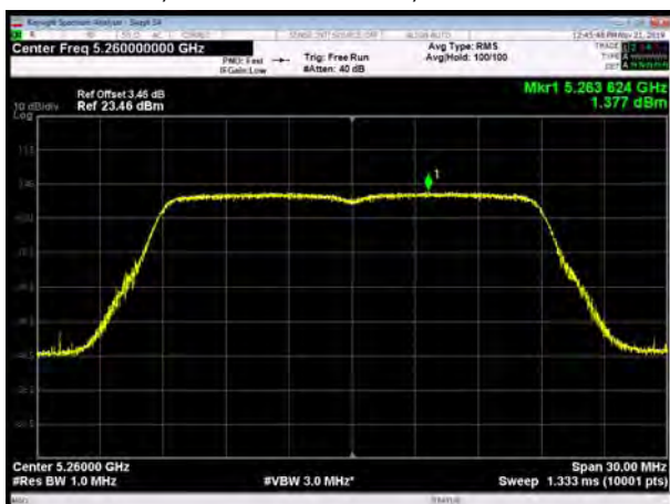
U-NII-2A, 802.11ac VHT20, Channel No.: 60
