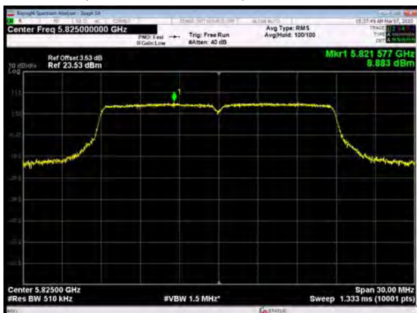
U-NII-3, 802.11ac VHT20, Channel No.: 165
