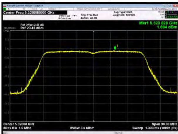
U-NII-2A, 802.11ac VHT20, Channel No.: 64
