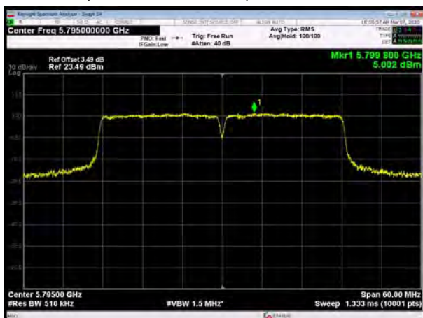
U-NII-3, 802.11ac VHT80, Channel No.: 155
