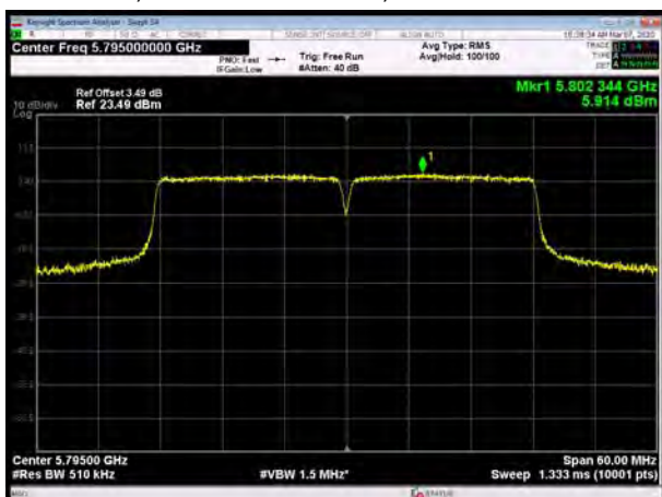
U-NII-3, 802.11ac VHT80, Channel No.: 155
