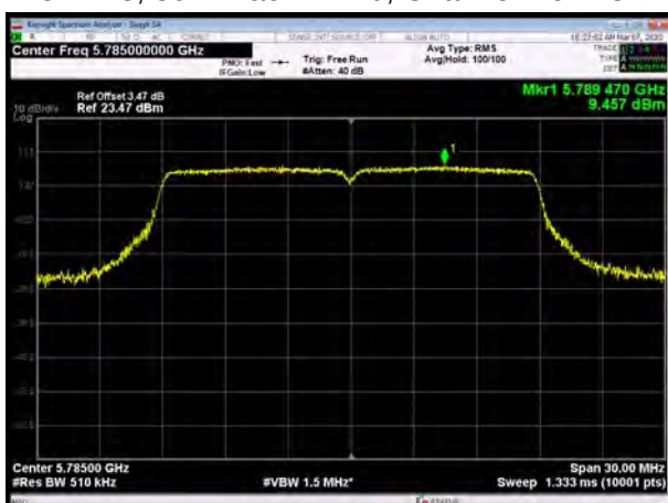
U-NII-3, 802.11ac VHT20, Channel No.: 165
