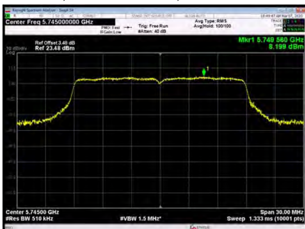
U-NII-3, 802.11ac VHT20, Channel No.: 157
