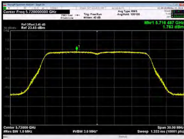
U-NII-2C, 802.11ac VHT80, Channel No.: 122
