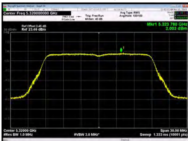
U-NII-2A, 802.11ac VHT20, Channel No.: 64
