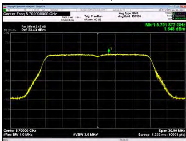
U-NII-2C, 802.11ac VHT20, Channel No.: 140
