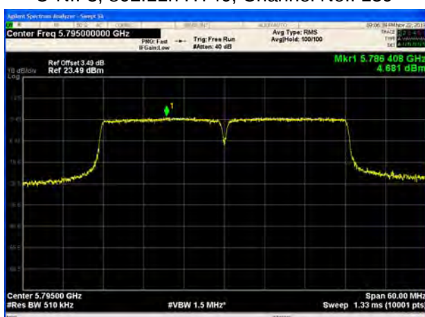
U-NII-3, 802.11ac VHT40, Channel No.: 151
