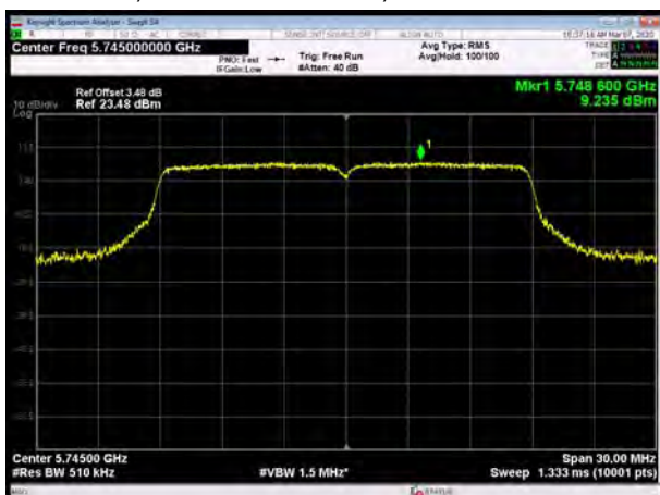
U-NII-3, 802.11ac VHT20, Channel No.: 157
