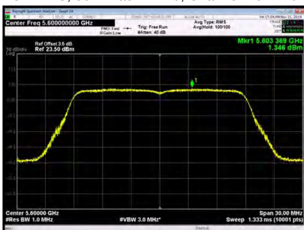
U-NII-2C, 802.11ac VHT20, Channel No.: 140
