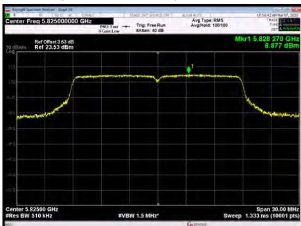
U-NII-3, 802.11ac VHT20, Channel No.: 165
